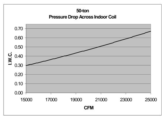
FIGURE 29 - 50 TON - PRESSURE DROP VS. CFM ACROSS INDOOR COIL
